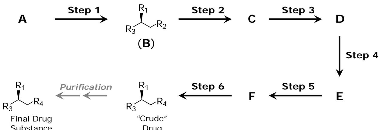
After the formation of intermediate **F** in Step 5, the mixture is heated to reflux. During reflux an impurity is formed through hydrolysis of intermediate **F**.
