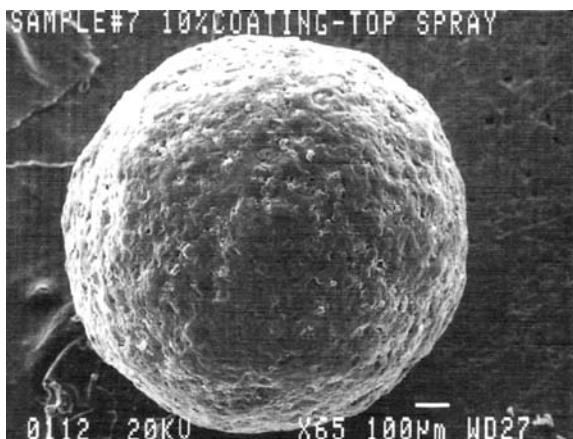
Figure 33 Surface view of PPA•HCl seed coated by top spray (granulating) method. Abbreviation: PPA, phenylpropanolamine.
