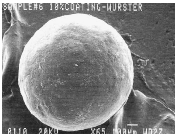
Figure 34 Surface view of PPA•HCl seed coated by Wurster method. Abbreviation: PPA, phenylpropanolamine.
