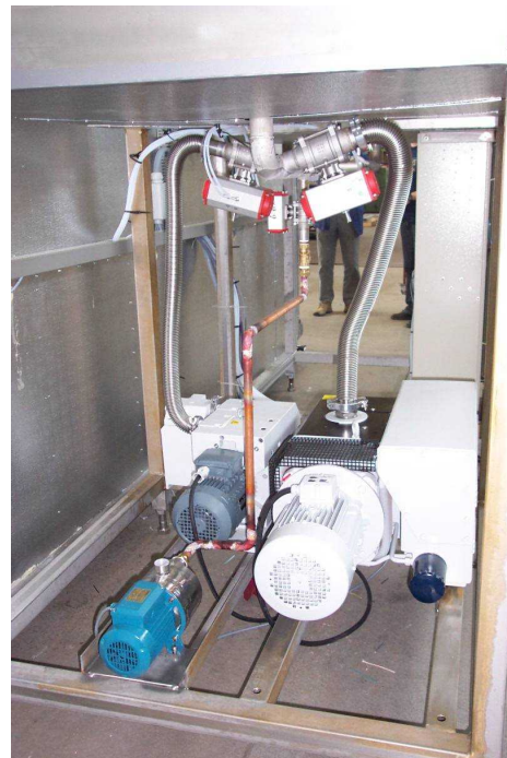
vacuum pump station , suction rate: 350m 3 /h
