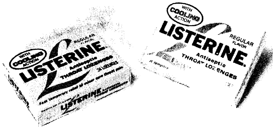
Figure 72 Carton overwrap. Moisture protection afforded the contents depends on the quality of seal and the moisture-transmission values of the wrap.
