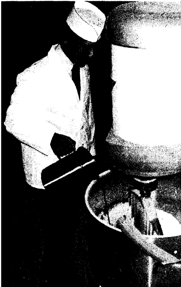
Figure 34 Preparation of flavor, medicament, acidulent, and ground salvage mixture as a master premix that can be subdivided into quantities suitable for incorporation into individual 100-lb. cooked candy base portions. The formulator is adding the flavor to the ground salvage, acidulent, and medicament mixture. This is followed by sufficient mixing to assure a uniform distribution throughout the batch. (Warner-Lambert Co.)
