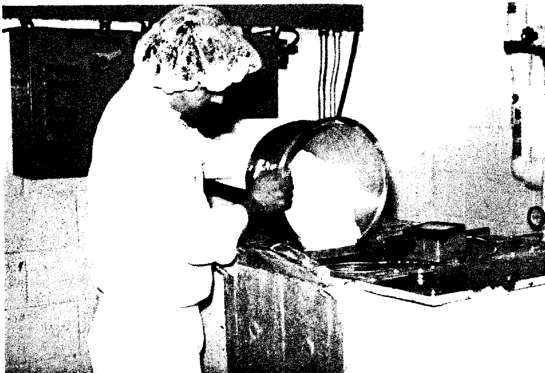
Figure 80 Flavor and seeding crystal addition. Seed should not be mixed for more than 10 minutes to avoid melting of the seed crystals into the batch. (Warner-Lambert Co.)
