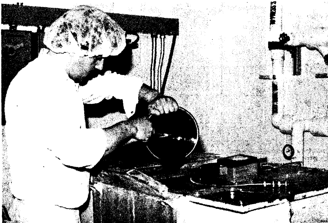
Figure 78 Color addition. Dyes are suspended in propylene glycol or glycerin to aid distribution. (Warner-Lambert Co.)
